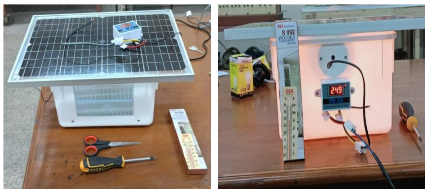
Figure 5. Thermostat Calibration Results with a Mercury Thermometer
