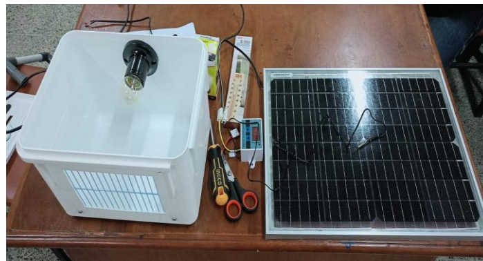
Figure 4. Thermostat-based 10-Egg Capacity Incubator with Photovoltaic Power Supply
